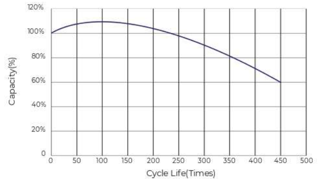
Cycle Life vs Remaining Capacity@25°C(77°F)
