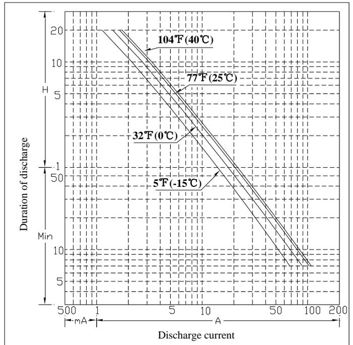
**Constant Current Discharge Rating Amperes @ 77 °F (25°C)**
